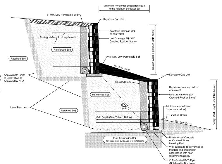
\*Note: Minimum wall embedment shall be 1.5 feet or greater to maintain the 1H:1V seperation between the bottom of the upper block wall and back of the lower block walls, as shown above.
